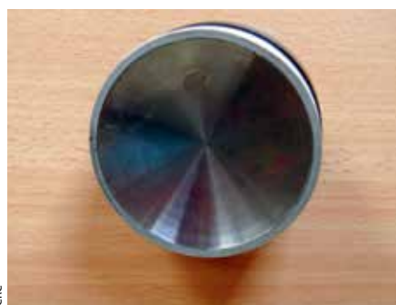
Figure A.7 Disc incorporated into an explosively-formed projectile.
